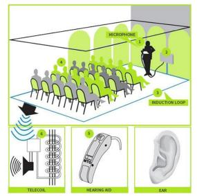
The 'loop' of cable generates a magnetic field signal throughout the area of coverage, transmitting the audio signal which can be received by the telecoil of hearing aids, cochlear implants and specific loop receiver devices with a T-Coil fitted.
